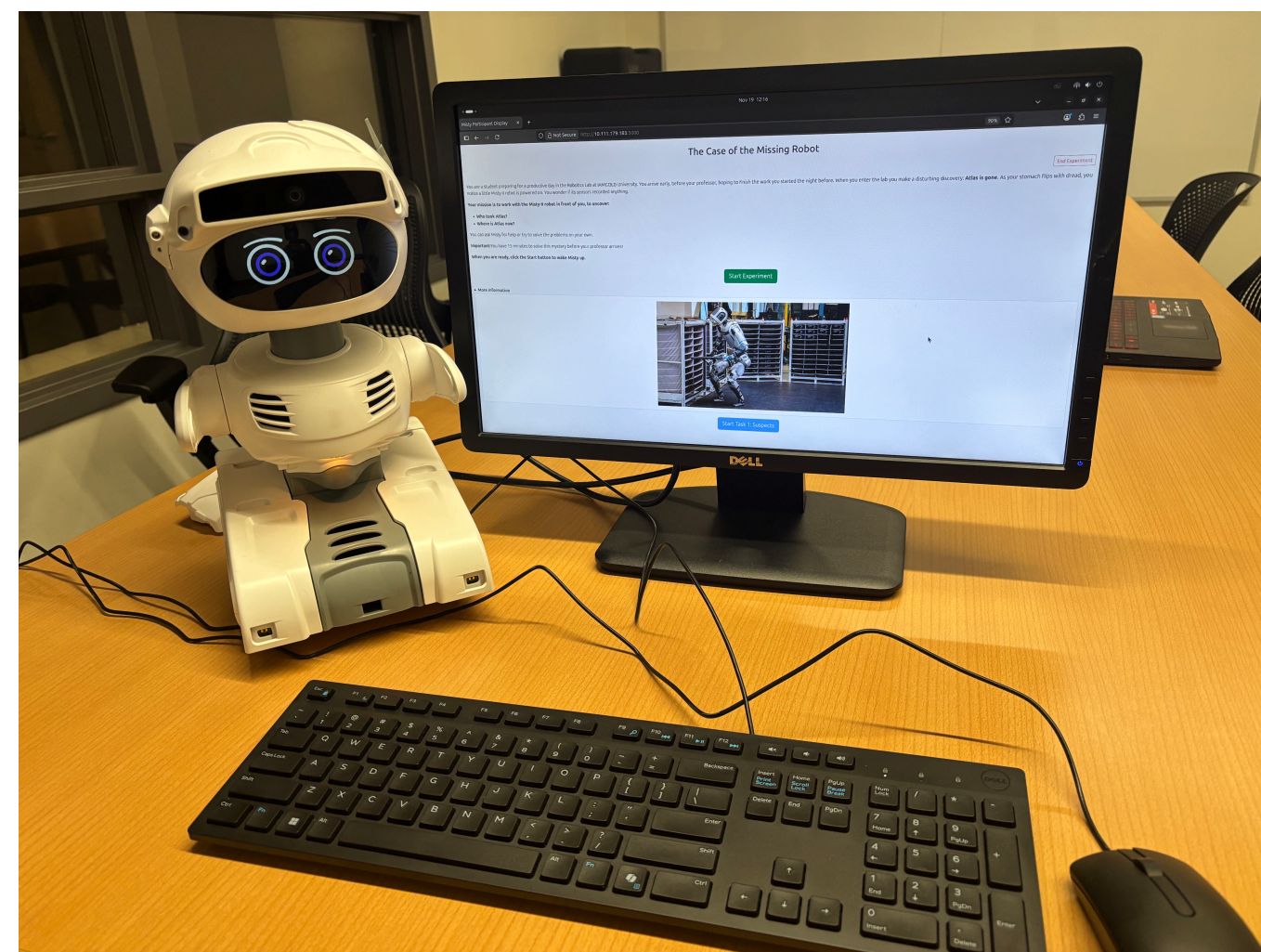
Figure 1: Experimental setup: Misty II social robot engaged in autonomous dialogue with a participant.
